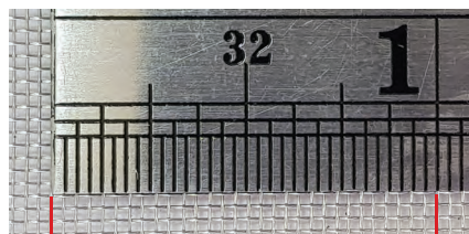
30 目：1英吋內有30個孔 30 mesh: 30 openings in one linear inch
